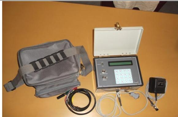
Systel Vibrating Wire Readout Box model SIS I-100 is a portable unit that is designed for the readout of all vibrating wire gages and transducers, and is capable of displaying the reading in digits, frequency (Hz), period ( $\mu$ s), or microstrain ( $\mu\epsilon$ ). The readout also displays the temperature of the transducer (embedded thermistor) with a resolution of 0.1°C. All readings can be transmitted to a host computer and imported into spreadsheet and database applications.
